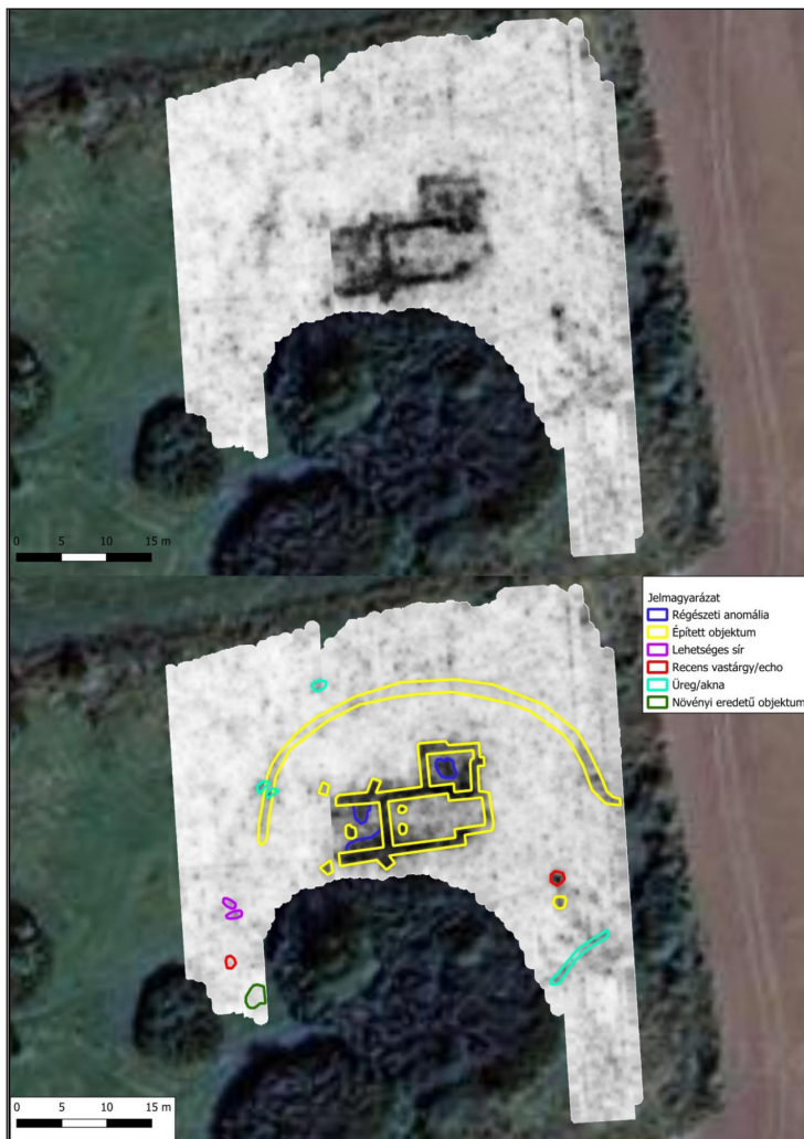
Fig. 5. GPR survey of the Varjaskér church area (-1 m depth slice map) with interpretation (by Máté Stibrányi, Munifex Ltd)
