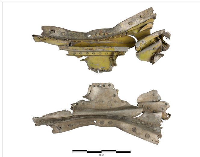
Fig. 3. A piece from the wing, clearly displaying the primer coating indicative of American manufacture (Photo: László György, Hungarian National Museum, National Archaeological Institute)
