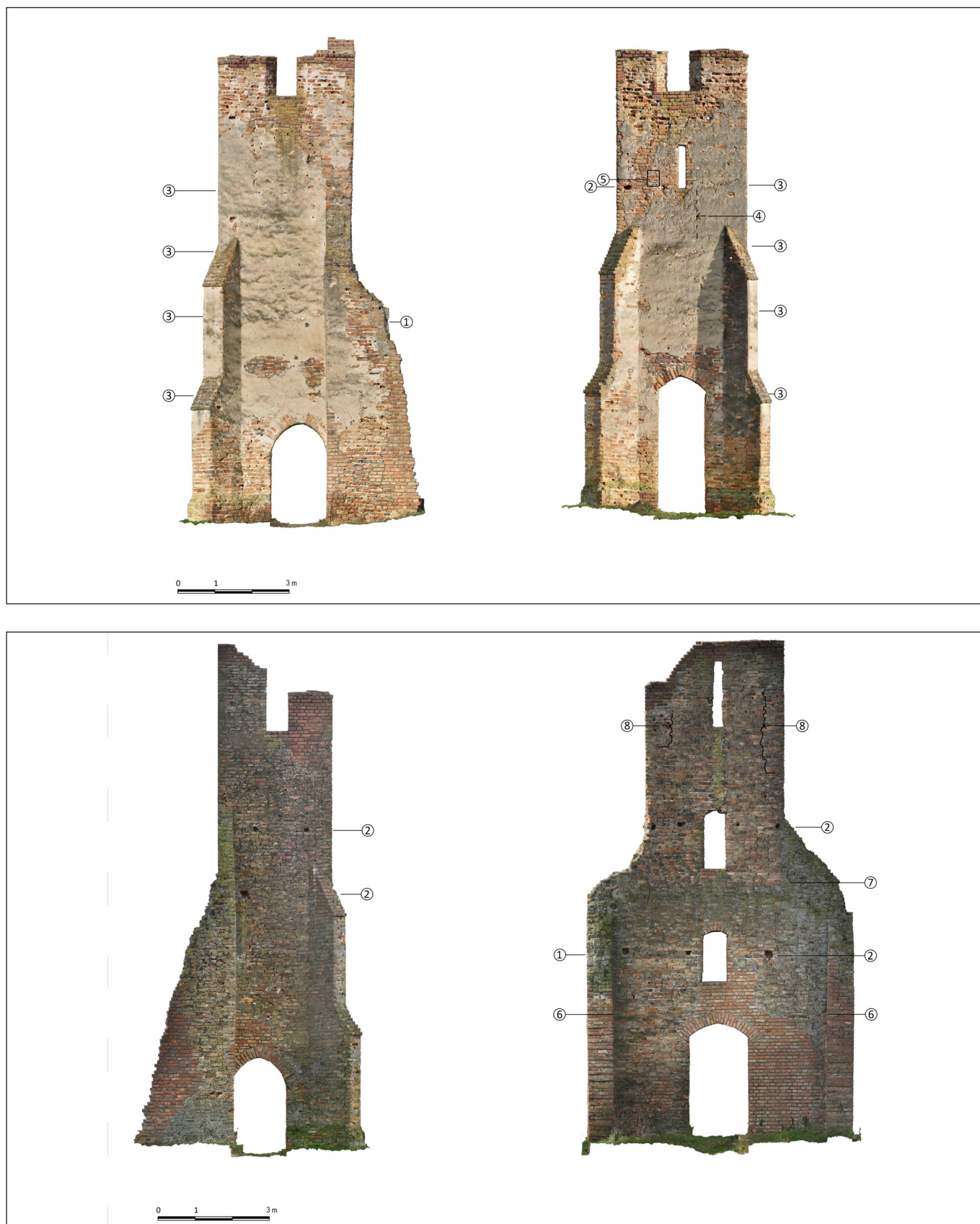
Figs. 3–4. Surveys of the tower's walls, 2025 (by Kvalitron Ltd, Tibor Szappanyos – KÖZTI cPLC). 1, Detail of a window frame and a window sill; 2, beam pockets of the scaffolding; 3, construction-related horizontal gaps in the plaster; 4, position of the construction-related gap on the inner wall face; 5, large beam pocket, perhaps for a lifting mechanism, likely bricked up during construction; 6, beam nests of the gallery in the corners of the two long walls; 7, a setback – the position of the ceiling; 8, construction-related joint in the wall. Arrow indicates the direction of the extension
