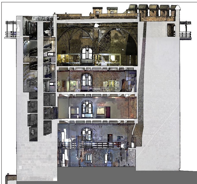
Fig. 2. Coloured point cloud longitudinal section of the Lower Castle of Visegrád, Salamon Tower
