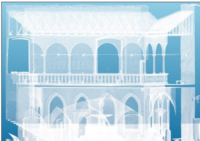
Fig. 5. Details of the Visegrád Royal Palace cloister in BIMcollab Zoom software, without displaying intensity values, and with highlighted edges
