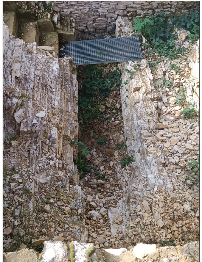
Fig. 5. Bottom of a mining trench with almost vertical limestone layers, the places where the rock was removed from, and the regrowing vegetation
