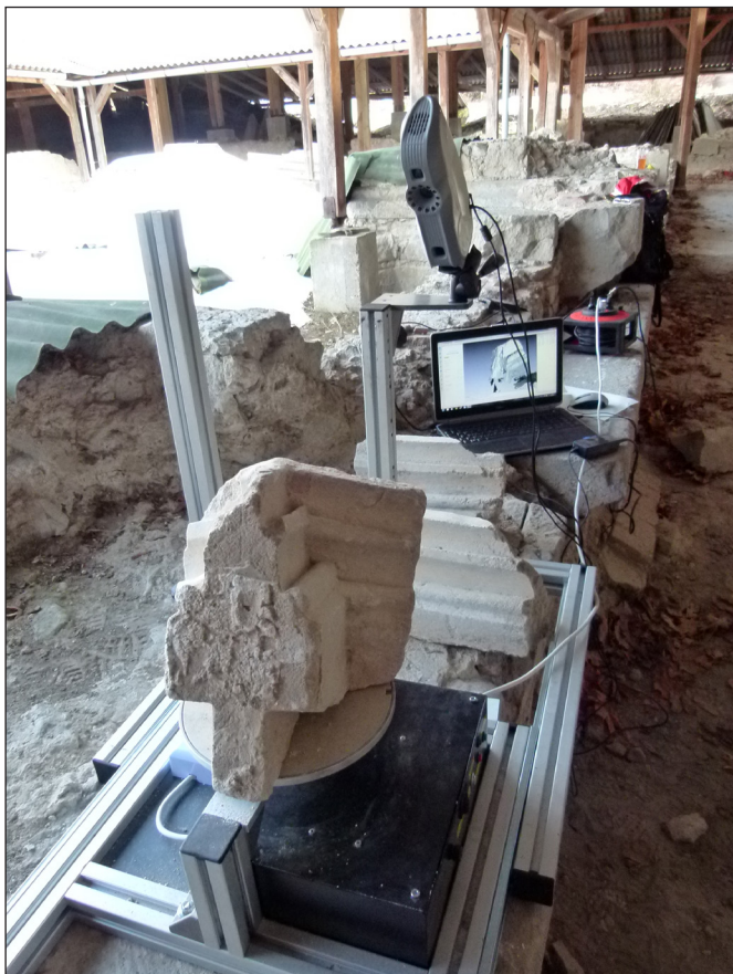
Fig. 16. Scanning the carved stones of the friary using an ‘Eva’ scanner and a rotary table, 2013 (photo by András Fehér)
