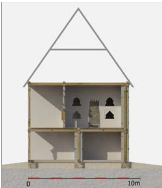
Fig. 15. Reconstructed cross-section of the palace building. Szolnok Castle, second half of the 16th century (3D model: B. Szőke)
