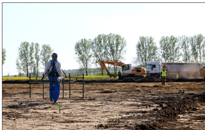
Fig. 3/1. Magnetometer survey of the topsoil-stripped surface
