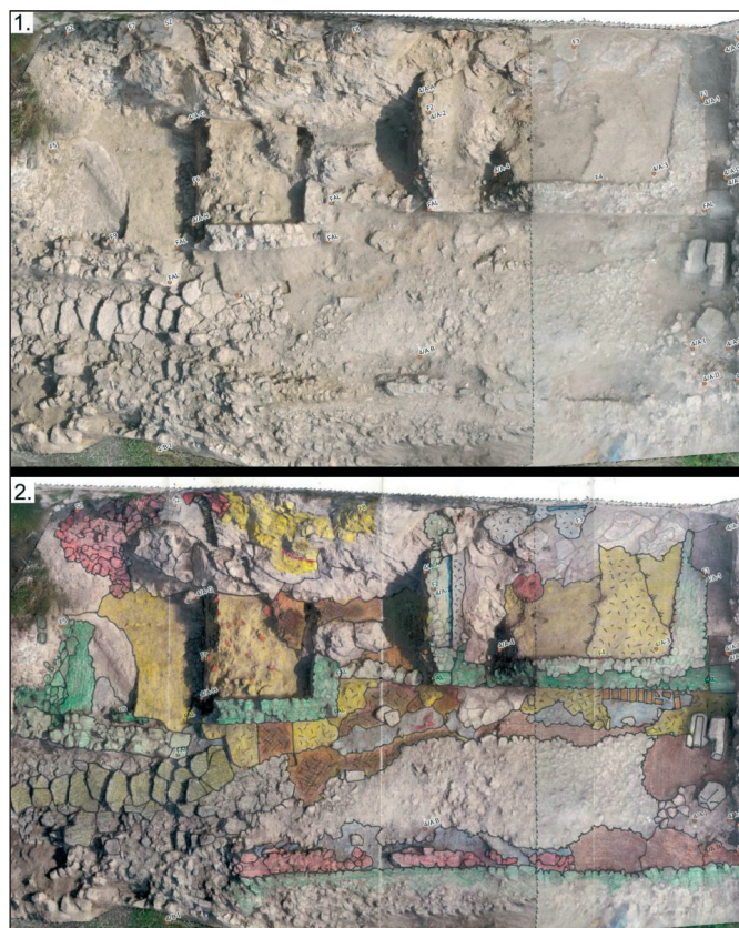
Fig. 5: 1.: Printable orthophoto made from a dense point cloud. 2.: Printed version drawn over with details recorded on-site (model: Krisztián Pokrovenszki, drawing: Gábor Hatházi)
