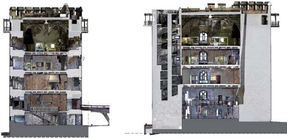
Figure 7. Cross-section layers with point cloud background
