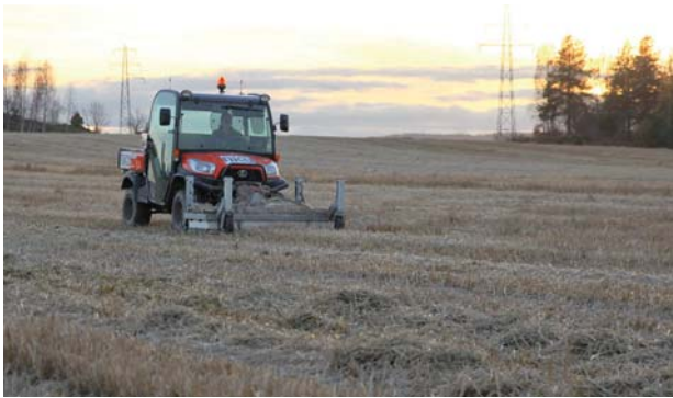
Figure 3. Large-scale prospecting GPR (photo: NIKU)
