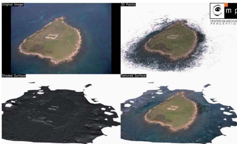
Figure 4. Surface model of the Croatian Island of Palacol derived from Structure from Motion (Image: Geert Verhoeven)
