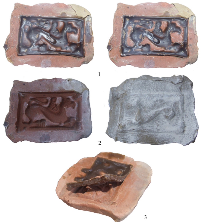
Fig. 4: Fired negative with the first model of even thickness. 1. Raw clay plaque, prepared for pressing against the reverse, 2. with the clay reverse, 3. removal of the wax model from the negative
