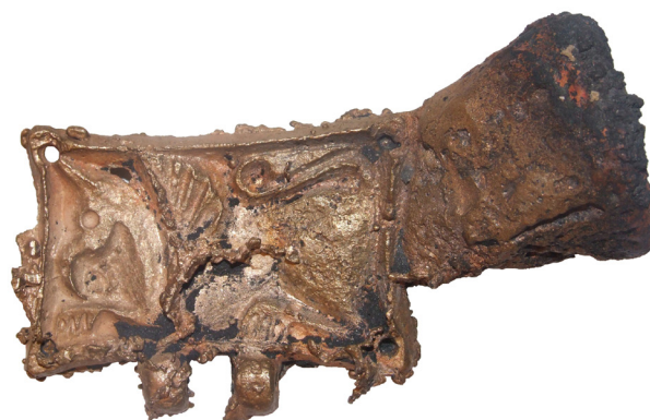
Fig. 12: Raw cast (flawed piece with casting seams and metal in the air bubbles of the mould)
