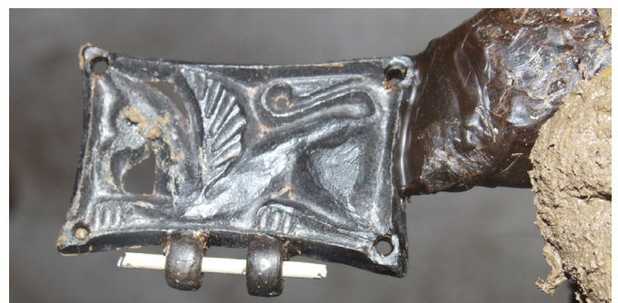
Fig. 6: The embellished wax model before embedding in the mould, with the wax model of the sprue and the clay-coated iron wire threaded through the hinges
