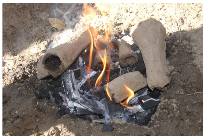
Fig. 9: Firing of the model in the furnace with charcoal fire used for smelting the metal
