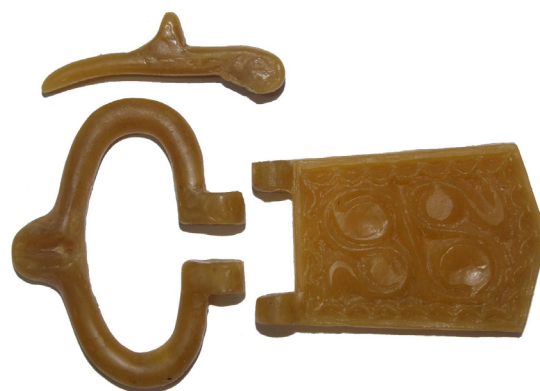
Fig. 3: Master model carved from beeswax: parts of a belt buckle
