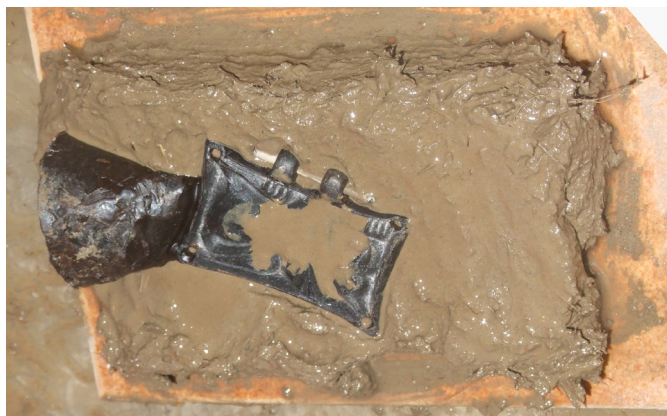
Fig. 7: The process of embedding the model
