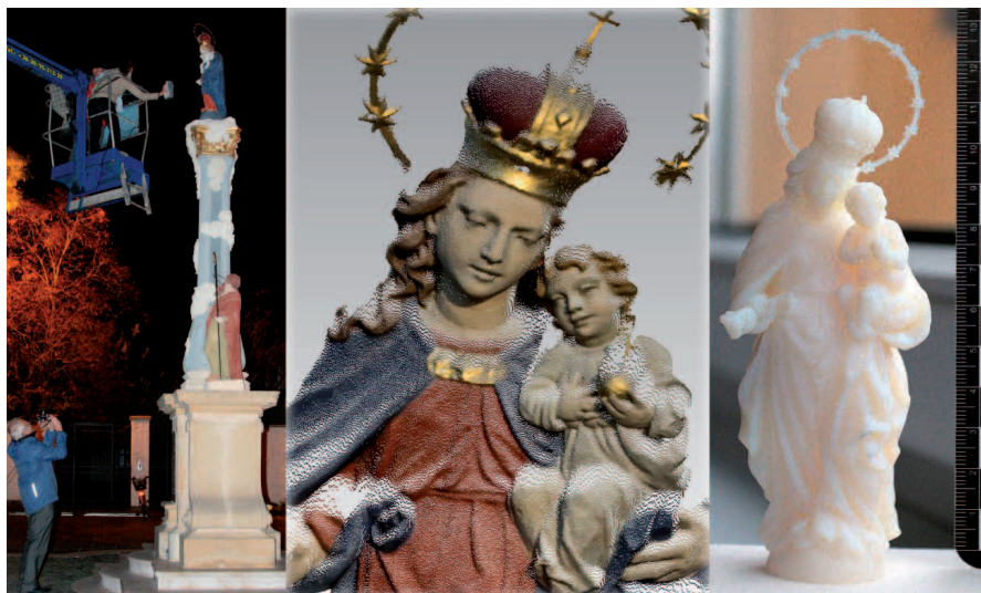
Fig. 6. Statue representing the Virgin Mary with the Child, Szeged. Object scanning (left), coloured point cloud of the terrestrial scanner (middle), 3D print of the sculpture (right).
