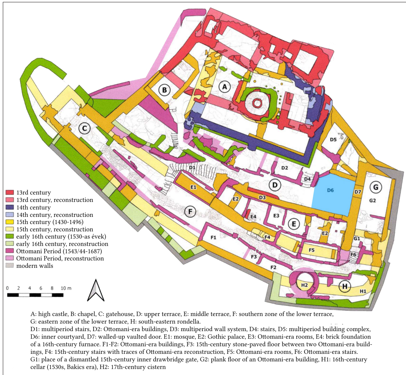
Fig. 2. Survey map of the Castle of Csókakő. The building phases are marked by colours; besides, the inner courtyard (D6) is highlighted in light blue (drawing by Balázs Holl, surveys by Balázs Holl, Krisztián Pokrovenszki, and Tamás Belegrai.
