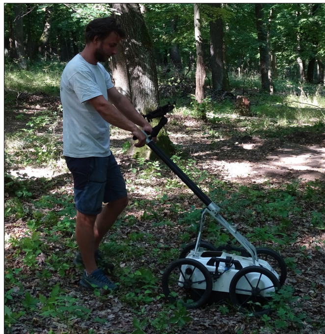
Fig. 5. Zsombor Klembala from the CH PLC carries out georadar survey on the site (photo by László Schilling)
