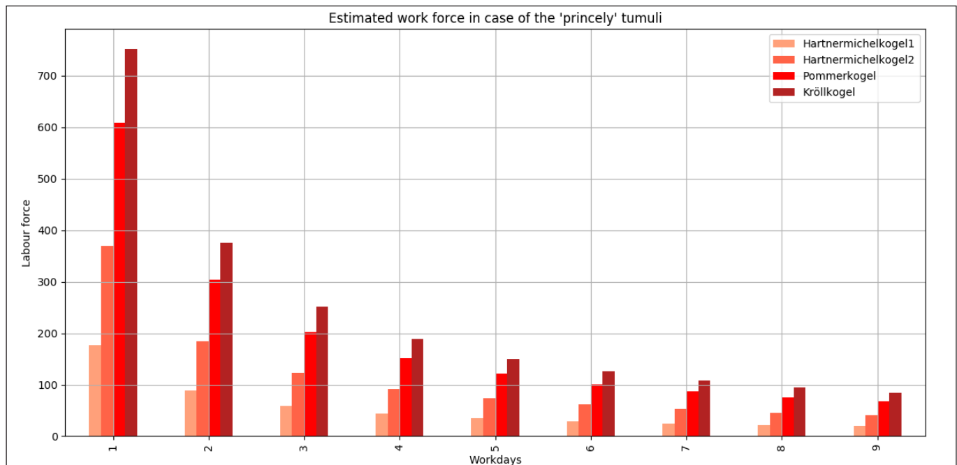
Fig. 4. The number of labour force necessary for construction of 'princely' mounds at Kleinklein according to the available number of workdays 22
