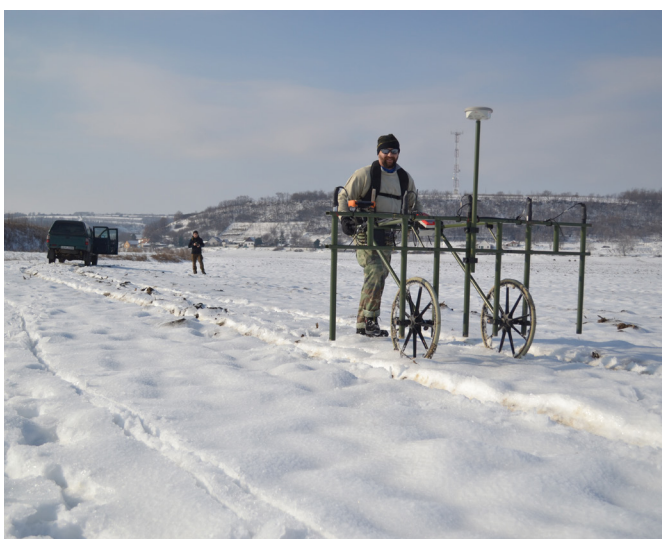
Fig. 3: The 5-channel magnetometer (SENSYS MAGNETO®-MX ARCH) in use (with Gábor Serlegi) at Alsónyék-Bátaszék. Sensors are placed at 50 cm intervals. (Photo: Knut Rassmann)
