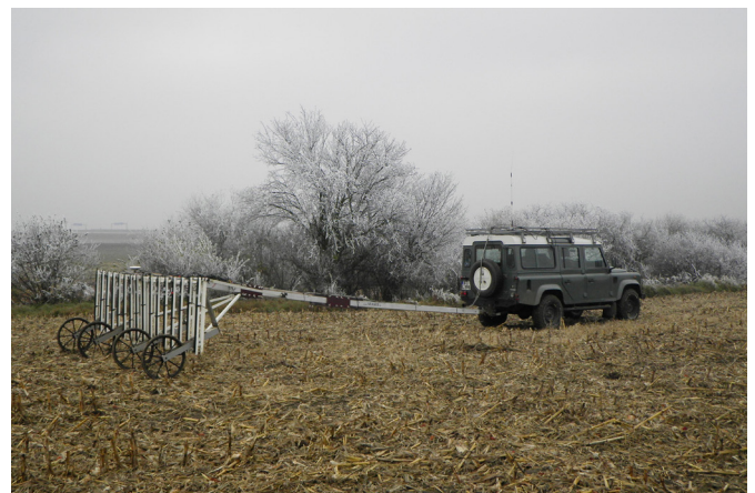
Fig. 2: The 16-channel magnetometer (SENSYS MAGNETO®-MX ARCH) at Tolna-Mözs (Photo: Kay Winkelmann)
