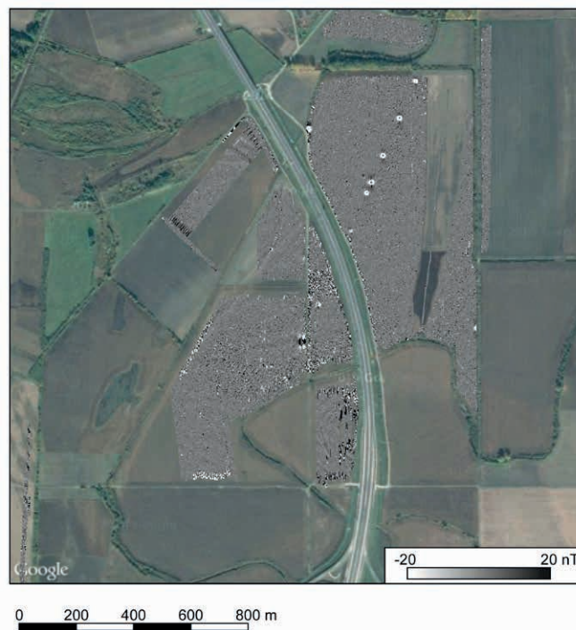
Fig. 3: Tolna-Möz, overview of geomagnetic prospection results from areas surveyed between 2011 and 2013 close to the M6 motorway
