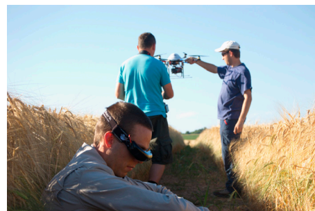
Fig. 8: Surveying a Roman villa with a multi-rotor copter. With the help of the transmitted live image viewable through the goggles the survey can be modified according to the needs of the specialists.
