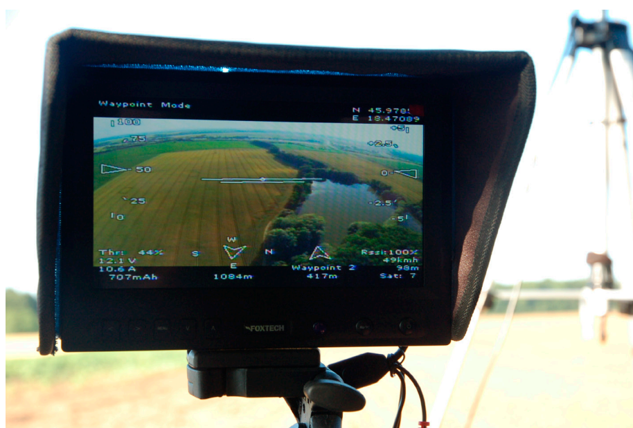
Fig. 10: Live video footage broadcast in mid-flight, containing the most important flight data as well
