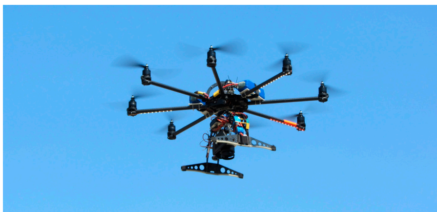
Fig. 7: Multi-rotor copter taking vertical photographs
